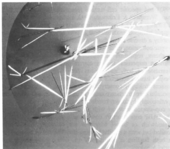
Fig. 2. Crystals of dimeric NGAL, photographed through crossed polarizers, grown from PEG at low pH. Average crystals grow to lengths of between 400 and 700 \mu\text{m} with widths of up to approximately 25 \mu\text{m} .
